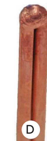
Figure 4. Blue laser copper welds, all void- and spatter-free. (a) A conduction mode weld. (b) A keyhole mode weld. (c) A butt weld for a bussbar. (d) A hairpin weld, as required for an ultra-compact electric motor assembly. Note that (c) and (d) are essentially impossible with alternative weld methods.
