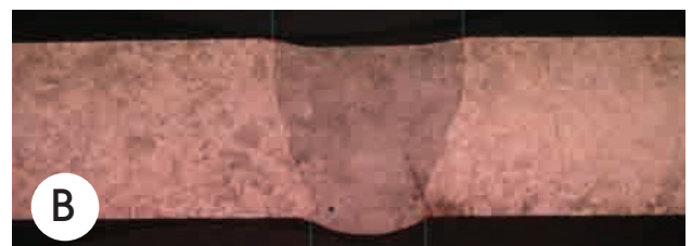
Figure 4. Blue laser copper welds, all void- and spatter-free. (a) A conduction mode weld. (b) A keyhole mode weld. (c) A butt weld for a bussbar. (d) A hairpin weld, as required for an ultra-compact electric motor assembly. Note that (c) and (d) are essentially impossible with alternative weld methods.
